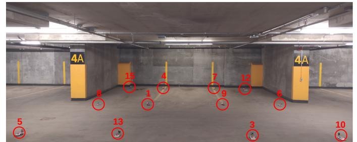
Fig. 17. Node distribution at the start of map construction experiments. Nodes are placed in a grid formation occupying an area around 8 m × 12 m.
