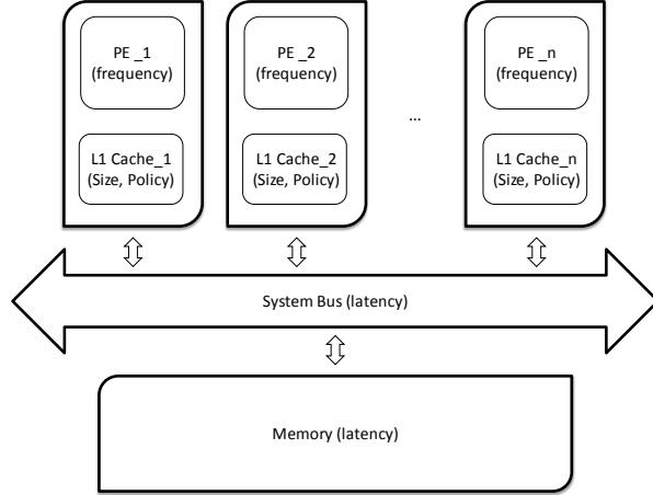
Fig. 1. The simulated multi-core processor architecture and its parameters.
